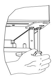
2. Remove corresponding screws on opposite side of cabinet. On some models there may be a nut behind one or both screws on either side.
