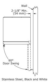
Units have a zero clearance for the door to open  $90^{\circ}$ , when installed adjacent to cabinets.
