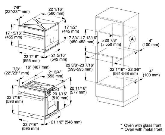
Cut-out (4" x 22" / 100 mm x 560 mm) in the bottom of the cabinet for power cord and ventilation
