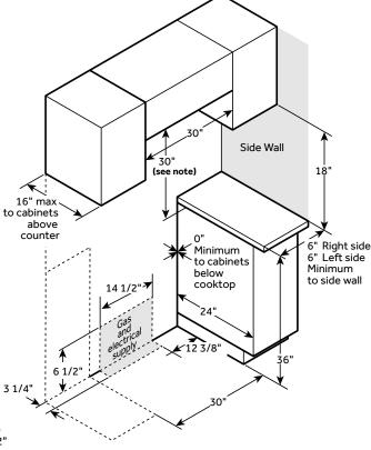
**Note:** Minimum to bare cabinet above; see Installation Instructions for alternate installation configurations.
