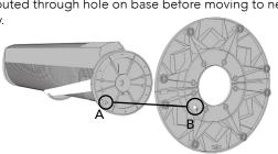
3. Attach base to tower using 8 screws provided.
