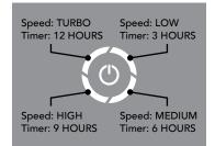
3. Press () to activate timer. The () and Indicator Lights will turn orange to indicate timer adjustment mode. While in this mode, select amount of time in three-hour intervals by pressing (). After a few seconds, the flashing orange Indicator Lights will turn white, indicating you have
