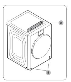
Using a level (A), check if the dryer is level side to side and then front to back. If the dryer is not level, turn the leveling feet (B) clockwise to lower the dryer or counterclockwise to raise the dryer.
