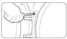
**9.** Place the door on the other side, and then reattach it to the dryer.
