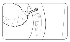
**11.** Re-attach the remaining screws to the remaining holes above and below the lever holder, and then tighten.
