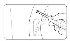
Remove the two screws above and below the lever holder on the opposite side of the door opening.
