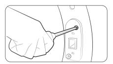
**10.** Push the lever holder into the cut out on the other side of the door opening. Insert screws, and then tighten as shown.
