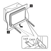
2 When the lower level is removed, remove from the upper two catches of the trim plate (5).
