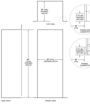
NOTE: 31/2" (89) finished returns will be visible and should be finished to match cabinetry
