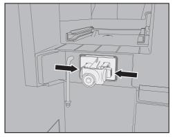
■ Press the catches on the left and right-hand sides of the milk valve holder and pull the holder forward to remove it.
