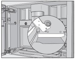
■ Clean the niche of the brew unit with a damp, clean cloth. Clean the areas marked in white in the illustration, e.g., around the drive shaft, especially well.
