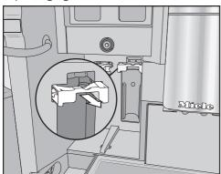
Pull the descaling cartridge holder forward.
