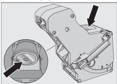
Wipe any remaining coffee off the two filters. One filter is located in the funnel and the other to the left of the funnel.
