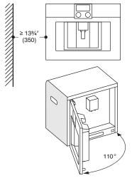
If using the 92  $^\circ$  door hinge restrictor (spare part no. 00636455), the minimum distance from the wall is only 4" (100).
