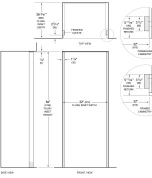
$NOTE: 3^{1}\!/z^*(89) \text{ finished returns and shaded areas will be visible and should be finished to match cabinetry Shaded line represents profile of unit <math display="inline">\textbf{hr} i k / t^*(19) \text{ panel}.$
