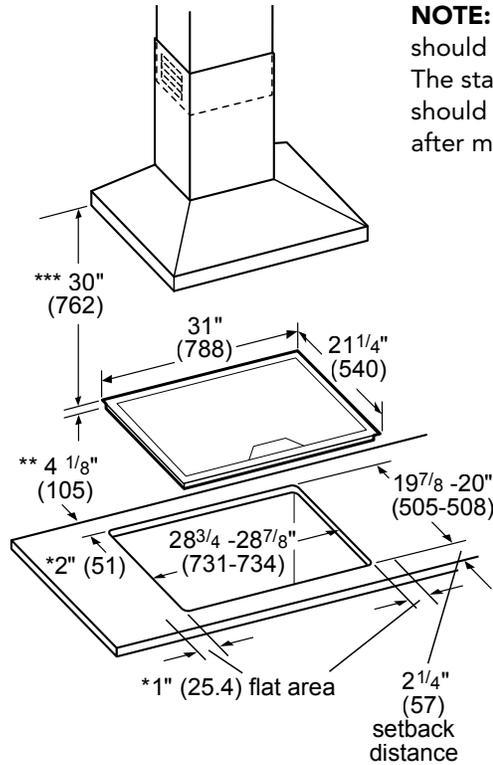
**NOTE:** The work surface should be horizontal and level. The stability of the countertop should be confirmed even after making the cutout.
