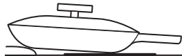
Pan bottom rests on cooktop trim or does not rest completely on the cooktop surface.
