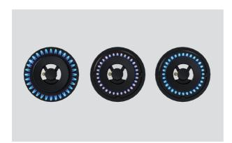
2. Check flames are blue and stable. A yellow flame indicates insufficient air. A noisy flame that lifts away from the burner indicates too much air.
