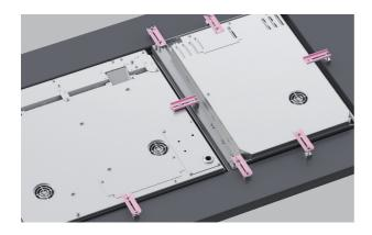
1. Fit the securing brackets to the base of each cooktop. For benchtops thinner than 25mm (1"), use the longer clamp screws.
