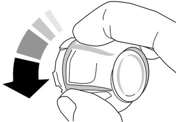
Locate the bulb cover and unscrew it by turning it counter-clockwise – it may be very stiff (**Fig. 6.2**).
