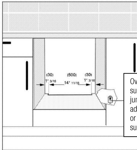
Oven electrical supply: Locate junction box in adjacent cabinet or below bottom support surface
