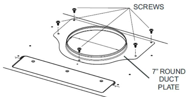
**TIP:** Insert a small length of duct over the 3¼"x 10" or 3¼"x14" damper assembly (for rectangular ducting) or 7" round (for round ducting) and seal the joint using aluminum foil duct tape to ease connection with the house ductwork.
