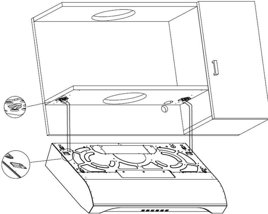
5. Fasten the hood by installing 4 pcs ST 3/16" x 11/16" screws (large flat head self tapping) into slots.
