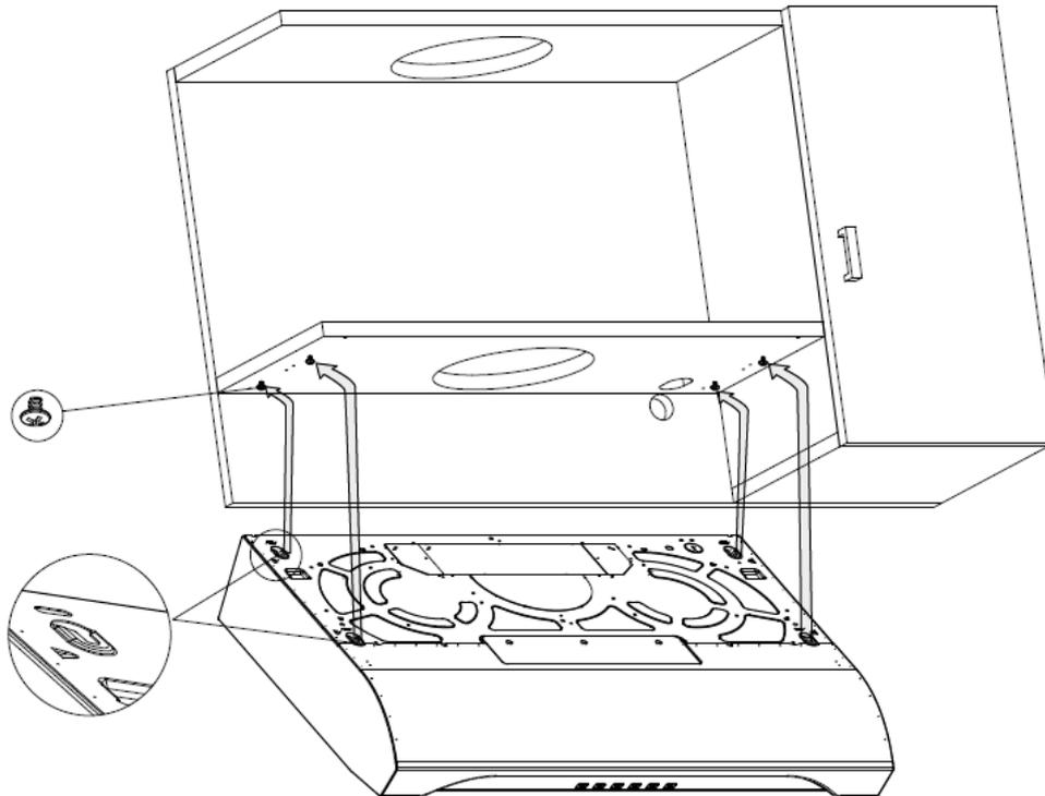
4. While holding the hood, run the house power cable into the hood through the strain relief previously installed.
