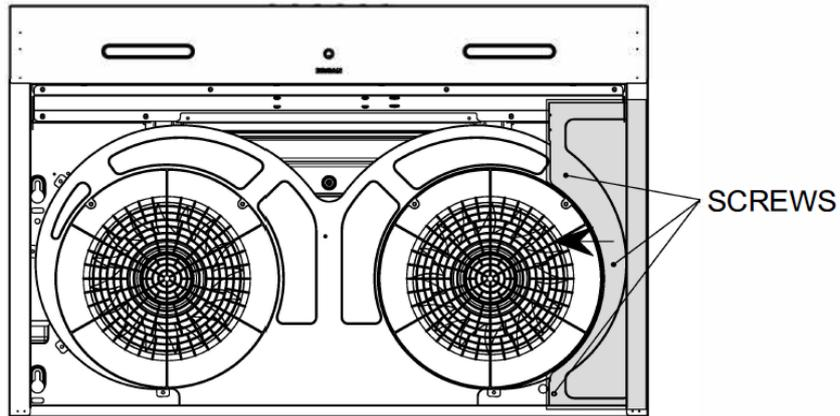
4. Use Phillips screwdriver to remove the 3 screws on the 7" round duct. Take off the 7" round duct.
