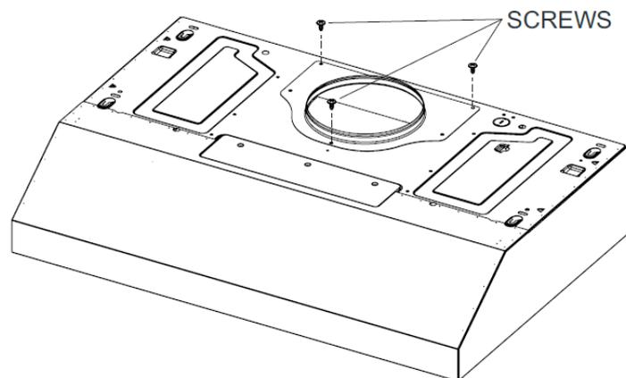
5. Remove electrical power cable knockout from top (vertical exhaust) or back (horizontal exhaust) of hood. For knockout removed from back of hood, install an appropriate strain relief, 1/2" diameter (not included).
