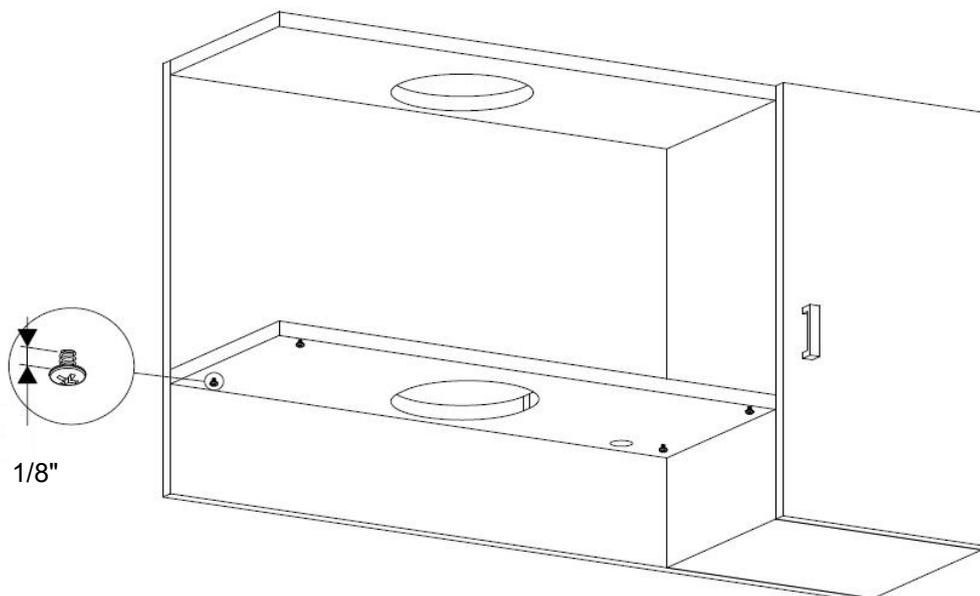
3. Lift the hood. Insert the 4 holes onto the screws. Slide the hood in place.
