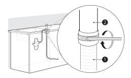
If it is not connected, attach the rubber hose connector to the disposal or waste tee with a hose clamp (not provided).
