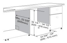
2 To allow for proper clearance of plumbing and electrical, use the template included with the literature to determine the clearance on the side of the cabinet where the cabinet meets the back wall. Using a 2 1/2" diameter hole saw, drill a hole in the target area as shown on the template.
