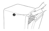
Align the dishwasher with the opening. Make sure the water supply line and power cord extend smoothly without kinks or bends.
