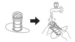
4 To replace the assembled filters, position the spray arm so the wider vee is toward the front. Fit the filters back into the filter holder and secure them by turning the inner filter clockwise until it clicks into place.
