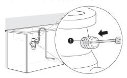
Remove the knockout plug from the disposal.
