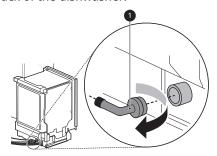
Connect the water supply tube to the elbow.
