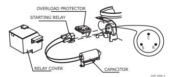
EMX20CLC Refrigerant R600a Voltage 115 - 127 VAC Frequency 60 Hz Run Cap 12µF/165 VAC Start Winding 6.7 Ohm at 77°F Run Winding 12.6 Ohm at 77°F LRA 3.7 A FLA 0.5 A Starting Device 8EA14C 4TM142RFBYY-53 Overload
