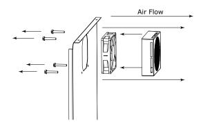
13.Remove and replace fan. Take special care to properly route fan wire.
