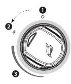
**Note:** If the magnet in the knob is disconnected, the indicator light will be orange. If the knob arrow is facing UP, gas is not flowing.
