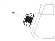
STEP 02 Use a Philips head screwdriver to remove the two (2) M4x10 screws from the knob bezel and set aside.
