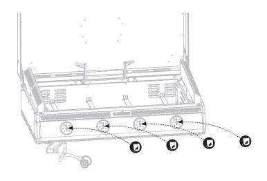
**STEP 04** Remove the four (4) protective washers from the griddle foot pins. With the help of another person, place the griddle top onto the griddle body by aligning the four foot pins to the holes on top of the unit.
