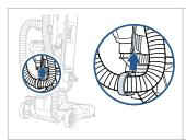
4. Attach hose clip to the body of the vacuum by clicking it into place.
