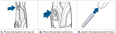
the hand vacuum handle and lightly pull to remove it from the machine.
