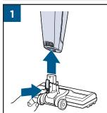
Make sure the vacuum is OFF. Press the release button to disconnect the removable floor nozzle from the hand vacuum.
