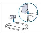
**1.** Align arrows on the storage tray with arrows on the brush roll drying tray and slide into place.
